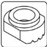
Ceramic Ferrule Chamfered for Round Anchors
