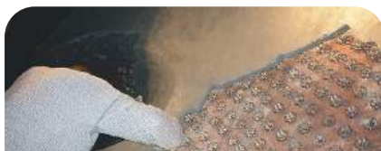
Installation of refractory onto SpeedCells®
